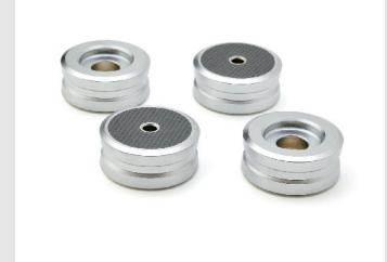
"INS-BS" is developed as an insulator which attenuates vibrations from a device and an installation surface and doesn't lose musical harmonics and dynamics. On one surface, there is a  $\phi$  20 4mm deep concave in which INS-CF can be set-in. This combination enhances Signal-to-Noise ratio and alters the timbre of the playback sound impression.
